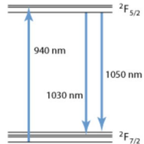
**Figure 1:** Energy levels of  $\text{Yb}^{3+}$  ions in  $\text{Yb}^{3+}:\text{YAG}$ , and the usual pump and **laser** transitions.
