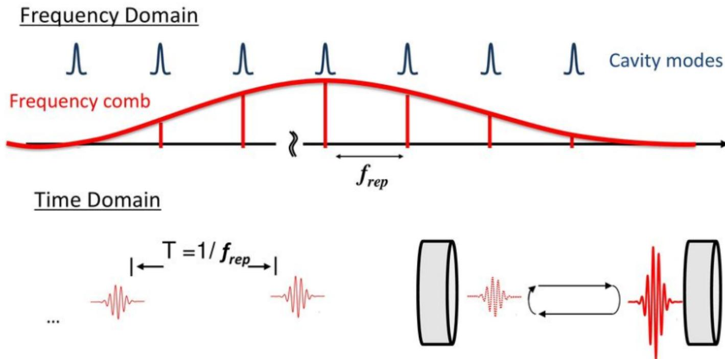
Finesse of  $> 1000$  with cavity enhancements of several hundred are possible with bandwidth  $\Delta\lambda \sim 30 \text{ nm}$
